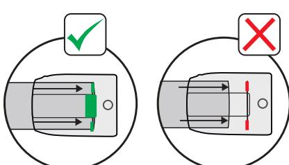
Insert the bevelled pipe end into the fitting until it stops and visually check the Green ring through the inspection window to ensure that the pipe is fully home. Minimum effort is required since all fittings contain silicone grease to make insertion easier.
