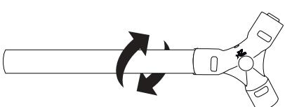
Bevel, and calibrate the pipe. Make sure that the pipe end has been bevelled both inner and outer layer all the edge long.
